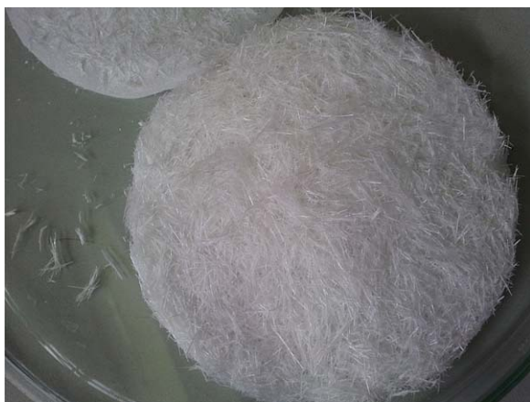
Figure 1. Washed and dried BHET synthesized from waste PET. [Color figure can be viewed in the online issue, which is available at wileyonlinelibrary.com .]
